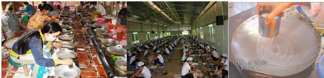
**Figure 2** Manual production process of net-wrappers [1]
