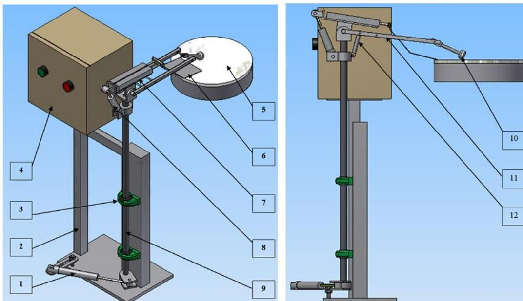
**Figure 6** The design of the pneumatic manipulator
