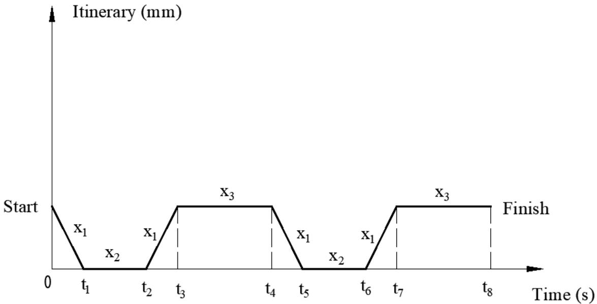
**Figure 9** Time chart of the manipulator's motion
