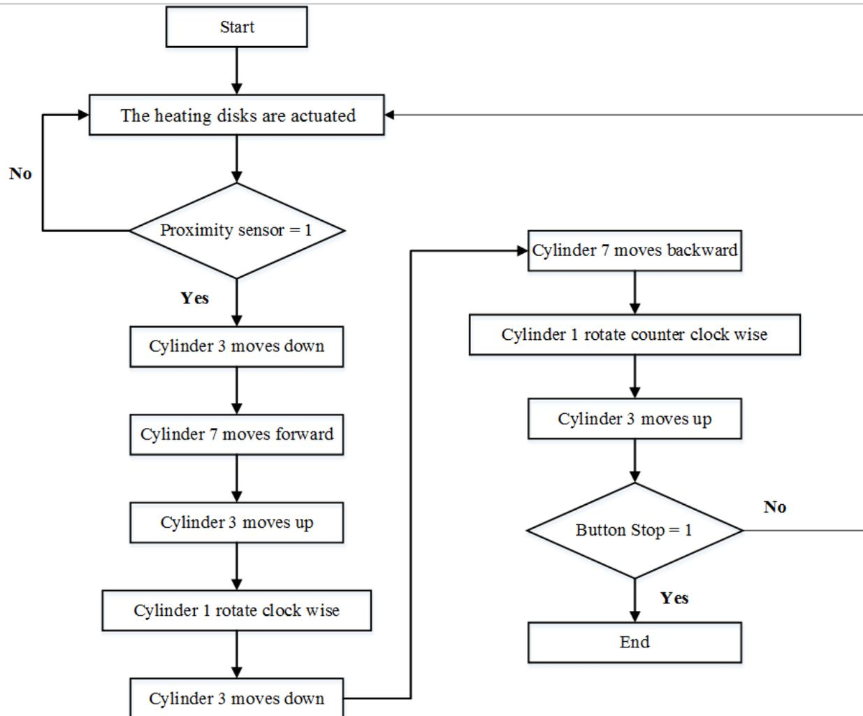
**Figure 8** Control algorithm for pneumatic manipulator
