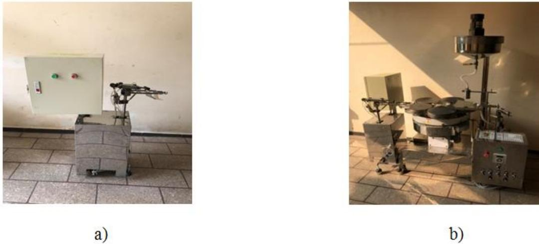
**Figure 11** a) Proposed manipulator prototype b) Manipulator is installed in semi-automatic machine
