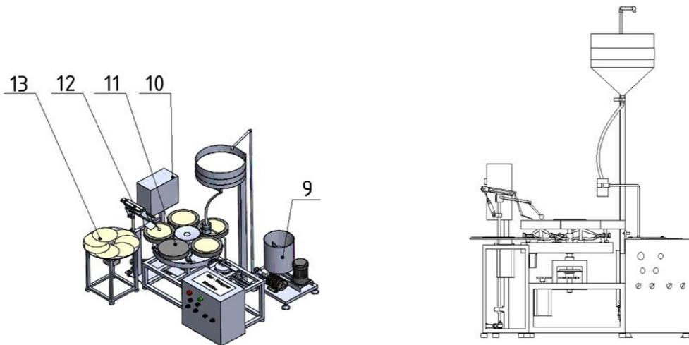
**Figure 5** Mechanism design with the manipulator arm for automatic net-wrapper removal.
