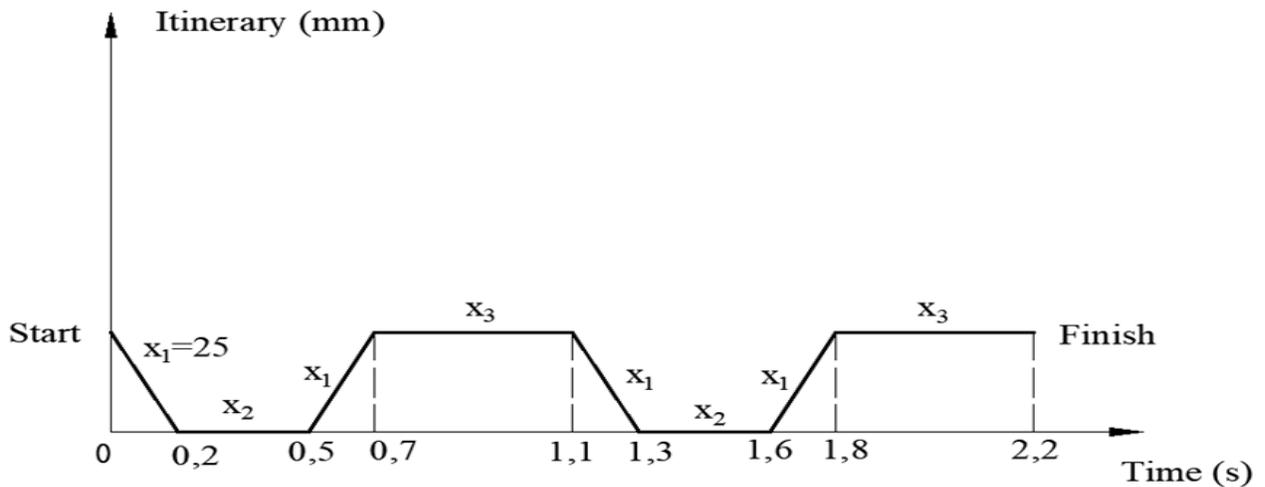
**Figure 12** Time chart of a manipulator arm for experimentation
