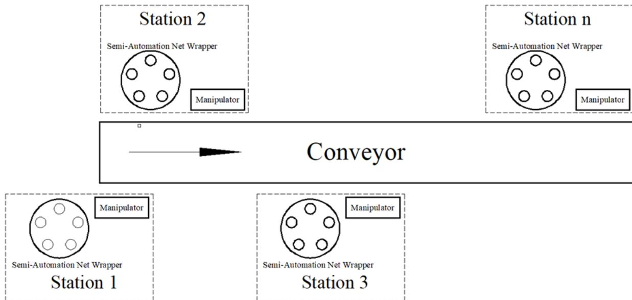
**Figure 10** Arrangement of the automated high productivity net wrapper system
