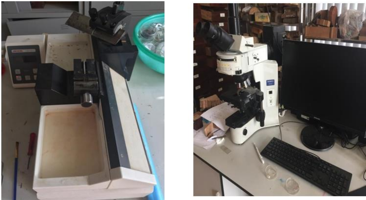
Figure 1. Cutting and capture devices to determine the wall thickness of the fiber cell
