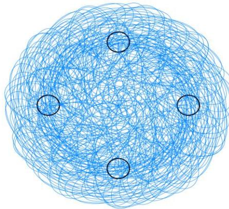
**Figure 2.** Net-wrapper shape and suction positions
