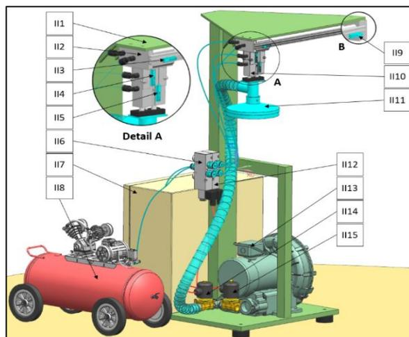
**Figure 6.** 3D model of the manipulator arm
