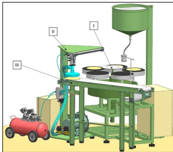
**Figure 5.** Layout diagram of equipment in spring rolls automatic production line.
