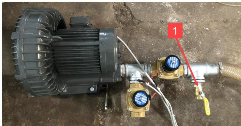
**Figure 10.** Solenoid valve arrangement to adjust pressure to suction head
