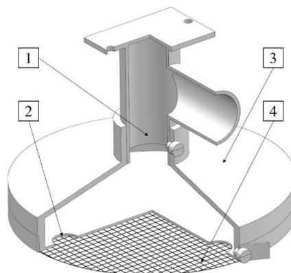
**Figure 3.** The suction funnel structure
