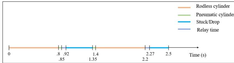
**Figure 9.** Time chart of the operation of manipulator arm
