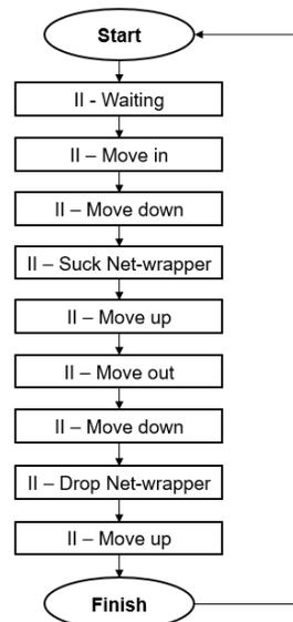
**Figure 7.** Block diagram of the operation principle of manipulator arm
