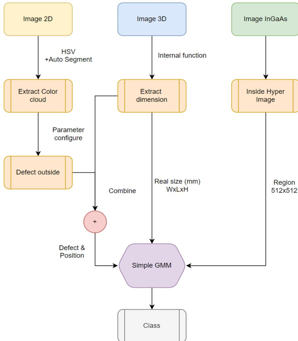
**Figure II-7** Process flow chart of the classification system
