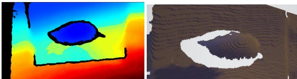
**Figure II-2** 3D point cloud image of the D435i. [6]
