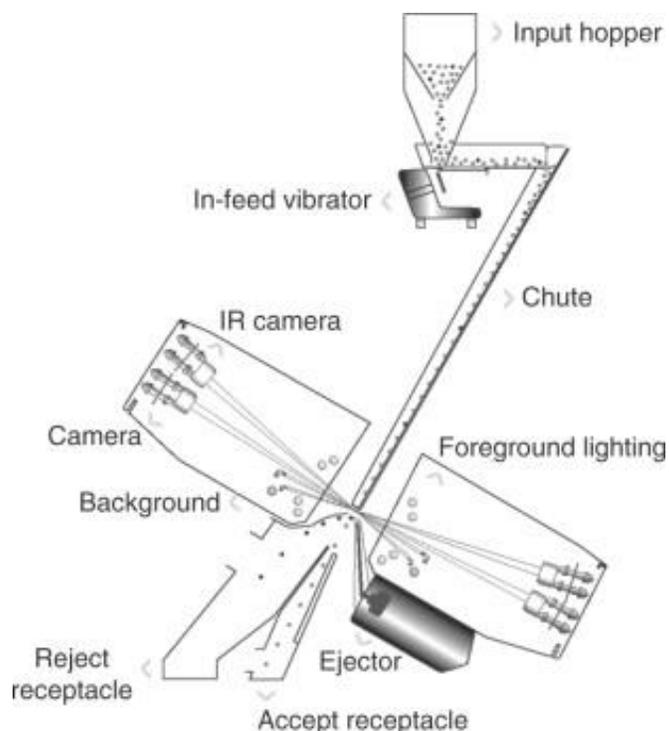
**Figure I-1** High-speed sorter using camera line [1]
