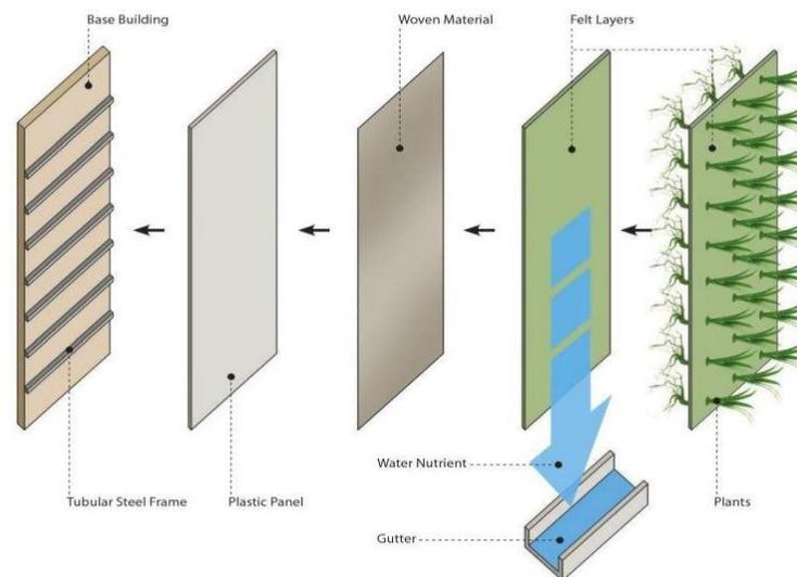
**Fig 14:** Exploded view of continuous LWS showing its irrigation
