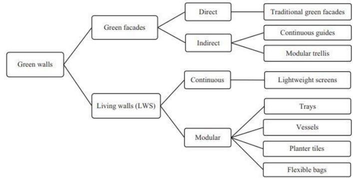
**Fig 1:** Classification of green walls based on construction characteristics (2)
